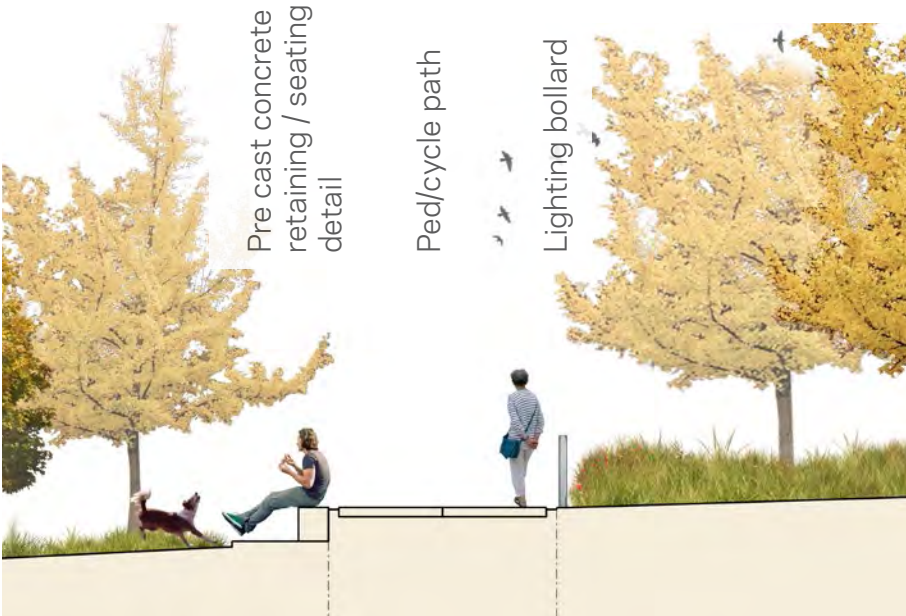
Detail through plot boundary interface
