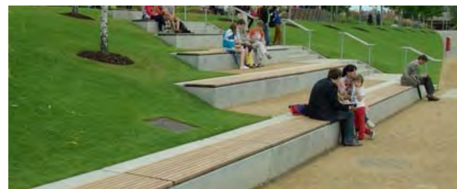
Public Realm Benches Hardwood slats on concrete base
